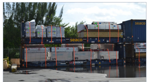
Properly strapped multilevel load.
